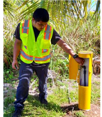
Each month, Rota operators collect samples from different areas of Rota to ensure the CUC Rota water is safe to drink. Here, Darien Rangamar, adjusts the flow of water from CUC Rota water sample tap before collecting a microbiological sample.
