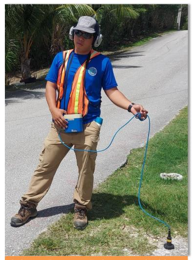
CUC Water Engineering Technician David Hidalgo listens for waterline leaks under a road. The ground microphone picks up and amplifies the sound of leaks. When a leak is found, the staff sprays paint on the road to mark the location so the repair crew can easily find the leak. Routine leak detection helps CUC protect the Saipan water resources and reduces water loss.
