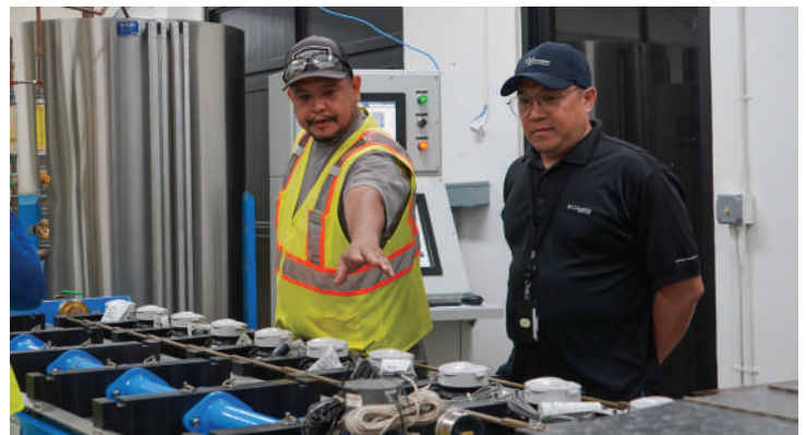
Joseph Robles and Christopher Deleon Guerrero demonstrate the water meter bench press, a tool used to test and calibrate water meters for accuracy before installation as part of the corporation's ongoing efforts to reduce Non-Revenue Water (NRW) by ensuring every drop is measured and accounted for.
